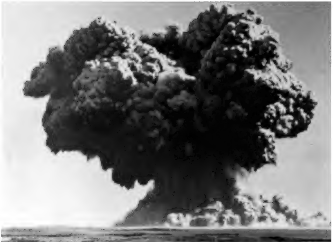
Fig. 3.8, cloud and base surge at 30 seconds. Water is falling from base of mushroom cloud at 65 ft/sec, and reached surface at 1 minute after burst. The base surge fallout was trivial.
